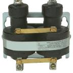
Tempco's Mercury Displacement Relays are specifically designed for resistive loads typical of heating and process equipment. These mercury relays are available in 35 and 60 amp models with single, double and triple pole configurations. Coil voltages range from 24 to 480 Volts AC at 50/60 Hz and 24 Volts DC.
