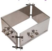
Hexagon shaped band heaters are used on the hex shaped portion of the nozzle on injection molding machines. These types of heaters are strictly made to customer specifications with bent-up flange clamping only.
