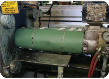
Tempco offers a line of Modular Insulating Blankets designed to contain the heat generated by industrial elements in various applications, thereby conserving energy and cooling the environment.
