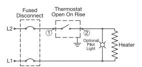
1Ø or 3Ø circuit if line voltage and/or current exceeds thermostat rating
