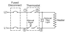
Typical circuit when voltage and/or line current does not exceed thermostat ratings
