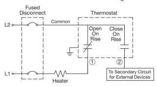
1Ø or 3Ø circuit if line voltage and/or current exceeds thermostat rating
