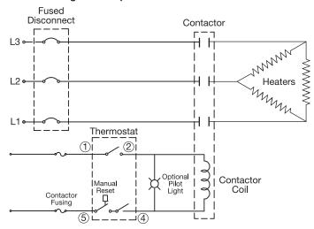
1Ø or 3Ø circuit if line voltage and/or current exceeds thermostat rating
