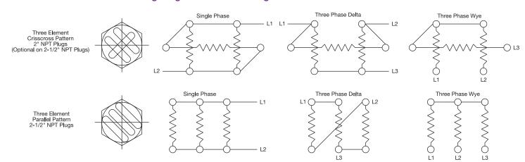
**NOTE:** Standard screw plug immersion heaters with three elements, factory wired for three-phase delta, can be rewired for single-phase operation with no wattage change. Wattage can be reduced to one-third of the designed wattage by switching from three-phase delta to wye connection.
