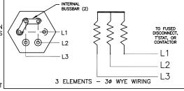
CAUTION! HEATERS DESIGNED & PRE-WIRED FOR THREE-PHASE WYE CAN NOT BE REWRED TO SINGLE-PHASE OR THREE-PHASE DELTA UTHOUT CAUSING PREMATURE HEATER FAILURE.
