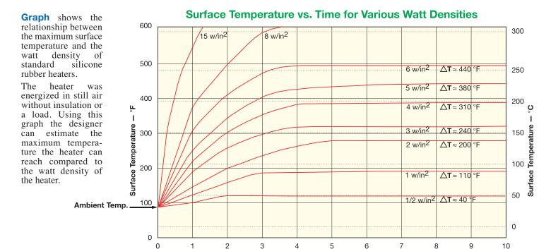
**△T** = Temperature Rise From Ambient at Specified Watt Densities
