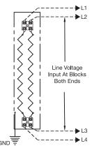
Double End Heater Wiring
