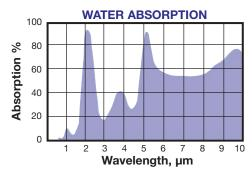
**SPECTRAL NATURE**: To address this issue, heaters should be designed to emit wavelengths that closely match the absorption band of the processed material in a given application. By carefully considering the broad side-bands of the emitted radiation and absorption, it is possible to design systems that will enhance the heat transfer rates at different stages of the heating process.
